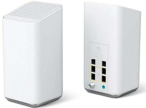
This is a picture of the rear of the XB7. The coax connection on the bottom left will remain unconnected. The Ethernet cable from the ONU (above) will plug in to Port 4 of this device (the one with the red vertical bar.) That leaves 3 “hardwired” ports plus two VoIP “POTS” telephone lines if you use that service from Comcast. Best practice is to place the XB7 near the ONU.
