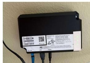
3. **White Cube Modem:** A new CAT 5e wire will be run from the ONU black box to a new white cube Modem. **You can have the modem installed anywhere you would like as long as it is physically possible.** You should expect wired speeds above 800 Mbps for upload and download. Wireless speeds will depend on the distance and walls from the modem.
